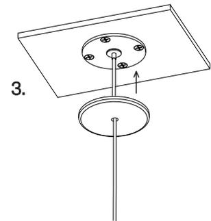
3. Screw the threaded cover plate onto the mounting plate.
