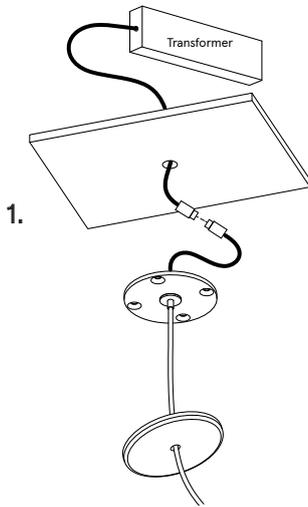
1. Prep the ceiling with an approx. 15mm hole. Place the transformer in the ceiling and feed the cable through the hole into the room. Connect the single electrified cable to the transformer.
