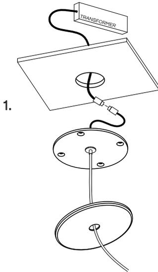
1. Prep the ceiling with a hole to suit the transformer size. Place the transformer in the ceiling and connect the single electrified cable to the transformer.
