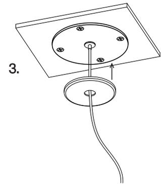
3. Screw the threaded cover plate onto the mounting plate.
