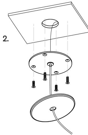
2. Screw the mounting plate to the ceiling using appropriate fasteners for the ceiling substrate.
