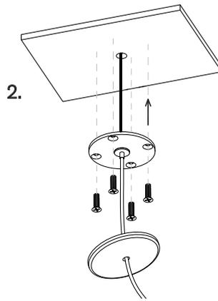
2. Screw the mounting plate to the ceiling using appropriate fasteners for the ceiling substrate.
