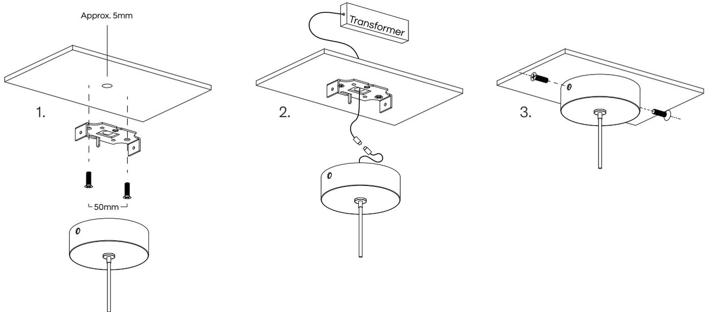
1. Fix the ceiling bracket to the ceiling using an appropriate fastener for the substrate. Prep the ceiling with an (approx. 5mm hole).
